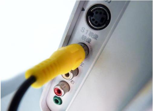
A close-up photograph of the yellow RCA connector of the AV cable being inserted into the AV input port of a television monitor. The port is labeled 'S1映像' and '映像'. | テレビモニターへ AV ケーブルを接続します。 |
